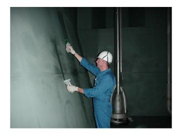
Firstly, and by design, the wall wash inspection is a random process, because it is impossible to write a procedure that exactly and precisely defines which places of a cargo tank should be "wallwashed"; particularly when no two cargo tanks are the same.
