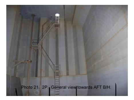
What these pictures clearly highlight is the fact that a wall wash inspection is really only representative of random parts of the lower 2 - 3M of any cargo tank. At best this equates to 10 - 15% of the internal surface area of the tank, but in reality, in terms of how much of the cargo tank is really wall washed, <u>it is significantly less than 1% of the total internal surface area of the cargo tank</u>.
